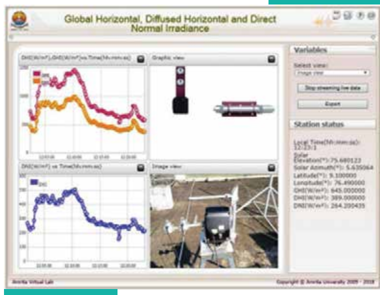
Figure 6: Screenshot of a remote triggered experiment on solar energy measurement
